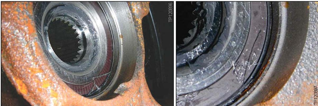
**NOTE:** Contamination on wheel speed sensor tone ring can cause intermittent errors.
